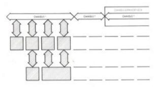
A full-blown PDP-8 system consists of many of each type of expansion device tied to the original OMNIBUS and its extensions. The basic -8/F and -8/M enclosures are smaller than that of the -8/E, and can accommodate only one OMNIBUS. Like the -8/E, however, an expander box can be added to bring the -8/F and -8/M capacity to 56 module slots.
