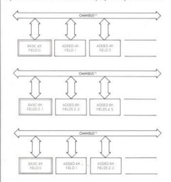
These diagrams illustrate some variations of memory expansion in the PDP-8. The basic 4K or 8K memory purchased with any PDP-8 is expanded, as required for expanded needs and added peripherals, in 4K or 8K increments up to a maximum of 32K words.
