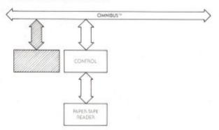
B. The second device type consists of a control module and an external peripheral instrument. The control module plugs into the OMNIBUS and links to the peripheral by cable. Multiple control modules may sometimes be required for this type of device also.
