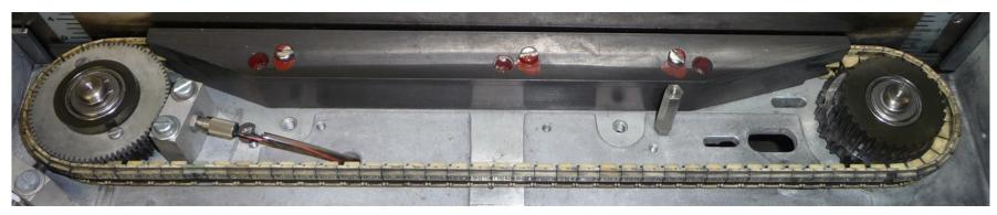
To print, hammers hit the paper against the ribbon when the correct character is under the hammer. This printer has 66 hammers which it moves back and forth to print the 132 print positions. This printer is the low end of the chain printer line. It only prints 125 lines per minute. High end printers would print over 1000 lines per minute.
